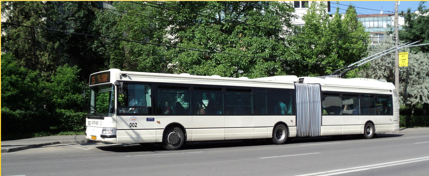
Articulated trolleybus obtained by modifying a diesel bus.
